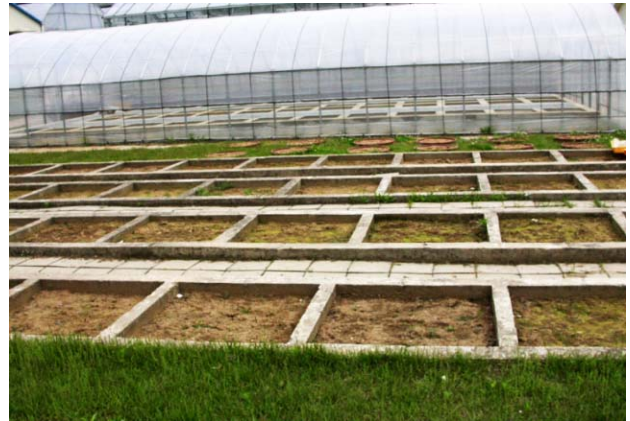
Fig. 1. Organic wastes-treated lysimeter applied with four different sludge wastes for eight consecutive years.
