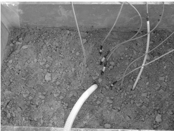
Fig. 12. PVDs and piezometer setup for model test box
