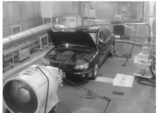
Photo. 1 Overview of chassis dynamometer
