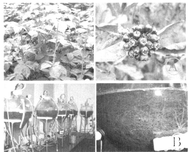
Figure 3. Plant and adventitious root production system for E. senticosus using bioreactor. A. Plant and seed of E. senticosus , B. Balloon type air-lift bioreactor culture of adventitious root of E. senticosus .
