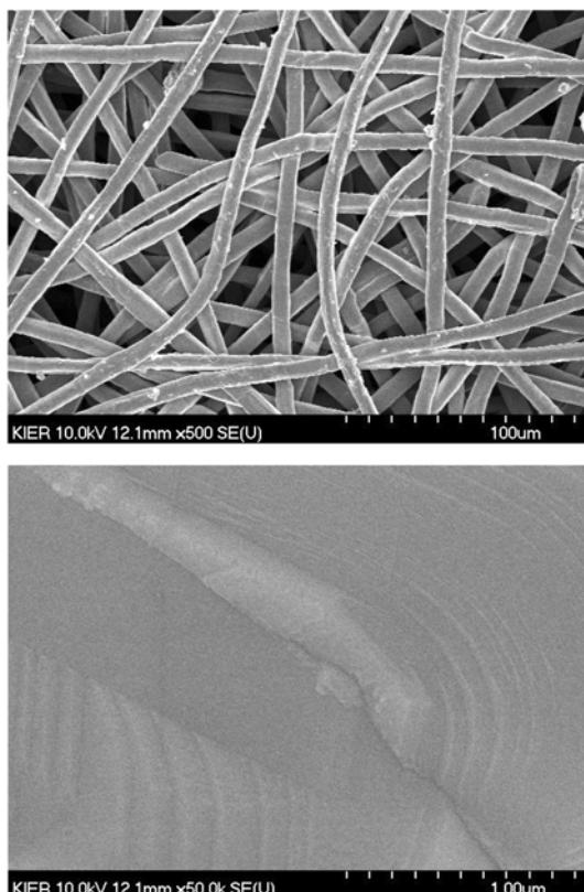
Fig. 1. SEM images of the micron-fibrous metal filter and its nascent surface.
