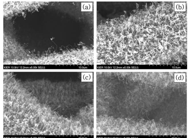
Fig. 3. SEM images of CNTs grown directly onto micron-fibers at several conditions such as (a) the  $C_2H_2$  flow rate of 5 sccm, (b) the Ar flow rate of 5 slm, (c) the synthesis temperature of 700 °C and (d) the synthesis time of 3 min.
