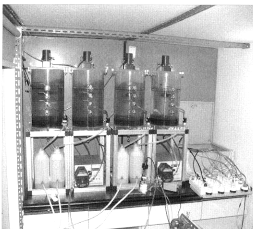
Fig. 1. Photograph and schematic of the lab scale SBR unit.
