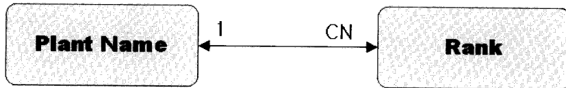
Fig. 1. Cardinality, entity relationship diagram: '1' means that a plant name has exactly 1 corresponding taxonomic rank. 'CN' means that every taxonomic rank is assigned to 0 to many plant names (Berendsohn, 1997)
