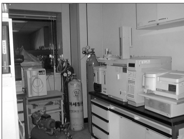
Figure 1. Unsecured acetylene and compressed gas cylinders in use
