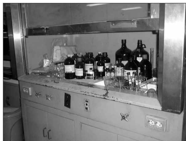
Figure 2. Storage of chemicals in fume hood
