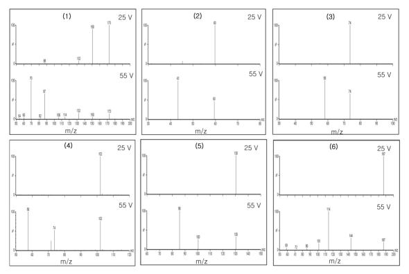
Fig. 2. Mass spectra of the standard amines and quaternary ammonium ions measured at the cone voltages of 25 and 55 V. Each solution of 10 μg/mL in water was introduced into the MS with a syringe pump. Compounds: (1) triethanolamine; (2) trimethylamine; (3) tetramethylammonium ion; (4) triethylamine; (5) tetraethylammonium ion; (6) tetrapropylammonium ion.
