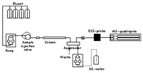
Fig. 1. Schematic diagram of the IC/ESI-MS system.
