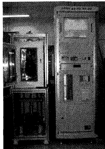
Figure 2. A schematic diagram and a picture of a newly developed test machine measuring the dimensional stability of rubbery materials upon temperature change: ① chamber, ② clamps, ③ load cell, ④ rod, ⑤ LVDT, ⑥ screw, ⑦ crosshead and ⑧ motor.
