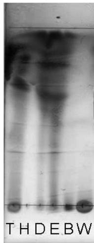
Fig. 4. Thin layer chromatography of various fractions of methanol extract of Curcuma rhizome T; total extract, H; n-hexane fraction, D; dichloromethane fraction, E; ethylacetate fraction, B; butanol fraction, and W; water fraction.
