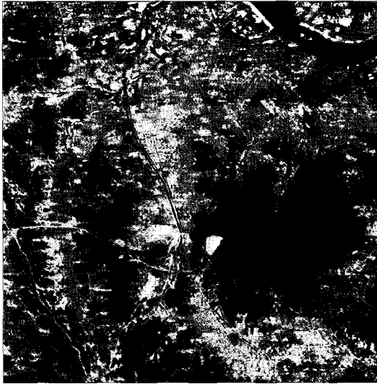
Fig. 5. Anaglyph of the southern Seoul area from Landsat stereomate using TIN interpolation.
