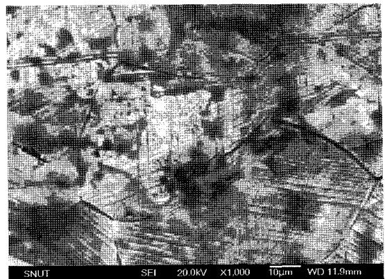
Fig. 9. Surface topography of a pin bushing bearing for a Diesel engine using a SEM.
