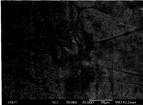
Fig. 7. Surface topography of an unlead based pin bushing bearing for a gasoline engine using a SEM.
