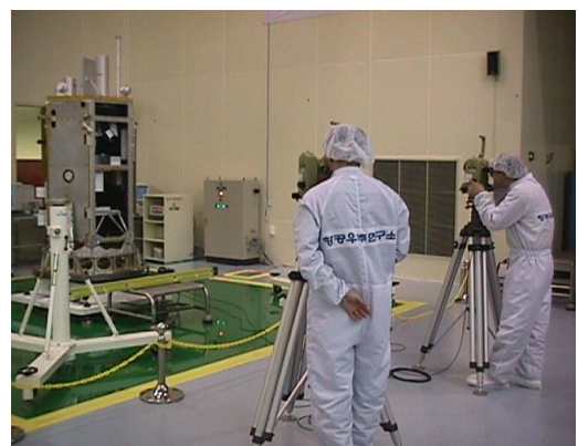
Fig. 2 3-D Measurement of Spacecraft Structure Model by Theodolite Measurement System
