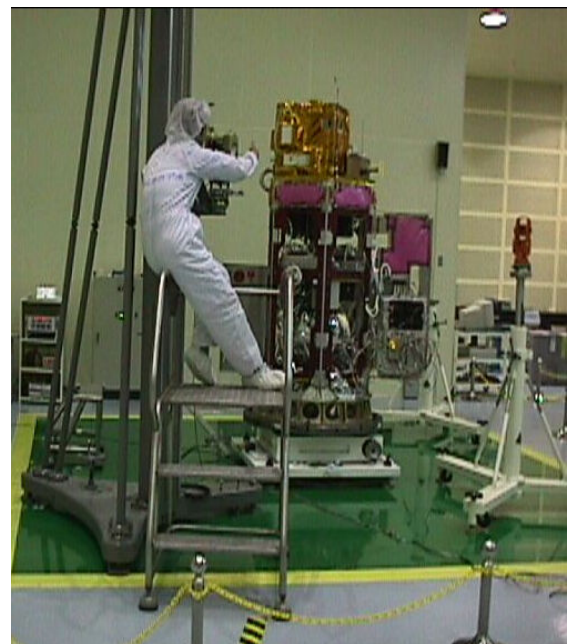
Fig. 10 Alignment Measurement of KOMPSAT 1
