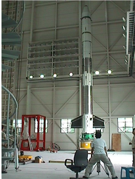
Fig. 3 Alignment Measurement for KSR-III
