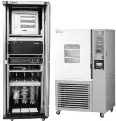
▲ PET Bottle CO 2 Retention Tester
