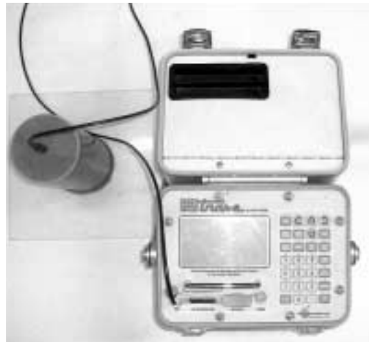
Fig. 3. Soil column & Trase-1 TDR
