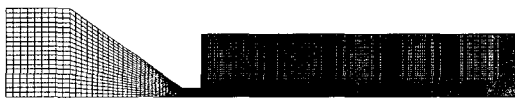
Fig. 1 Schematic of the problem configuration in axisymmetric drop ejection chamber and the grid system
