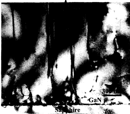
Fig. 5. Bright field image of defects in GaN grown along [0001] direction on the sapphire substrate used in this experiment. The beam direction is close to [1010] of GaN crystal.
