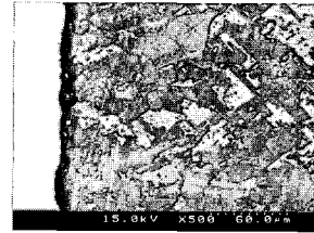
Fig. 4 Effect of Wire Cutting on Microstructure
