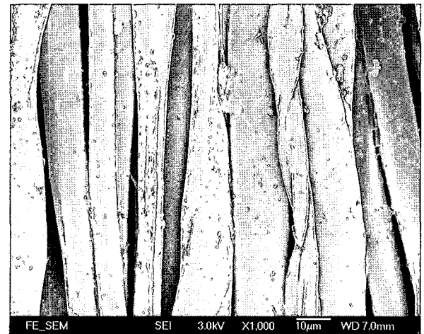
Figure 2. SEM image of MMT-treated fabric with no binder after 3 times of padding ( \times 1,000 ).
