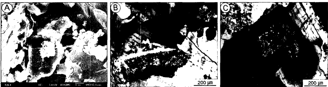
Fig. 2. Microphotographs for the rock properties of Mireuksaji stone pagoda. (A) Scanning electron microphotographs of rock-forming minerals, altered minerals and organic matters. (B, C) Rock-forming and alteration minerals showing host rock of the Mireuksaji pagoda.
