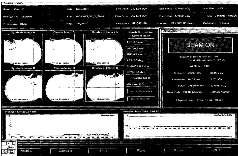
Fig. 3. X-rays showing cranial bony landmarks tracked continuously and simultaneously by use of real-time image guidance. The measured position as seen by both cameras is communicated through a real-time control loop to a robotic manipulator that redirects the beam to the intended target.
