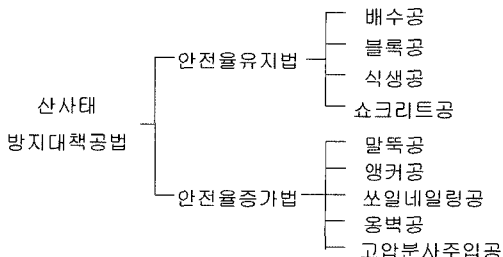
Fig. 6. Classification of the slope stabilization method in Korea (Hong & Song, 2002).
