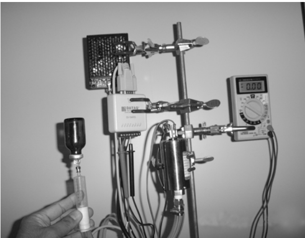
Fig. 1. A schematic picture of the pressure calcimeter system to determine soil inorganic carbon.
