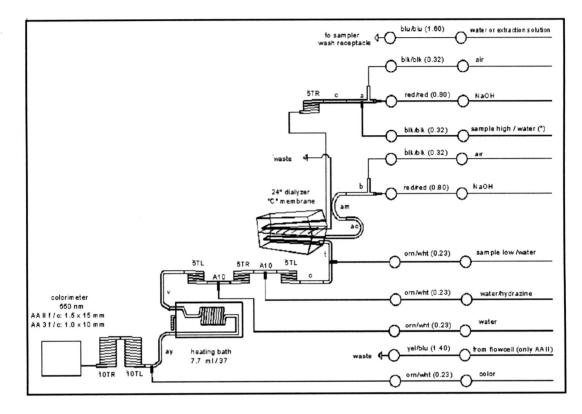
Fig 1. A diagram of the CFA instrument. (http://www.bran-luebbe.com)
