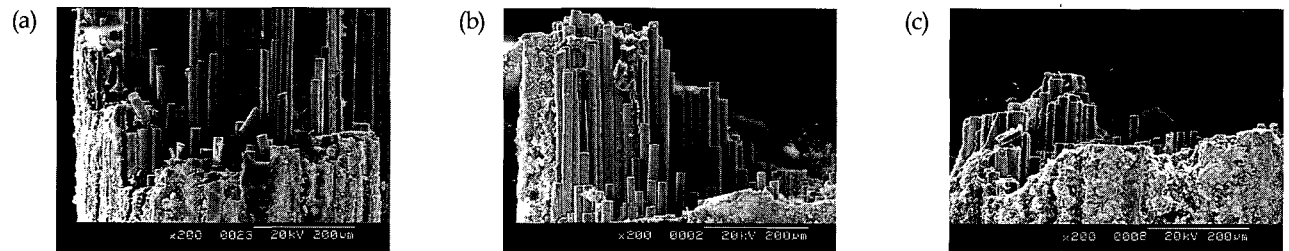
Fig. 9 SEM photographs of tensile fracture surface of E-glass fiber/vinylester resin composites as a function of immersion time in Alkaline solution environment at 80°C: (a) 5 days, (b) 60 days, (c) 150 days
