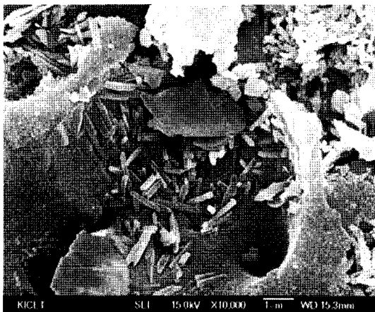
Fig. 17 Reaction products of fly ash mortar with NaOH+ water glass curing condition H1
