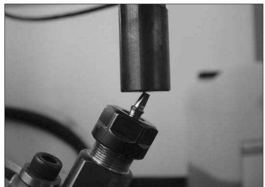
Fig. 2. Fatigue testing machine and jig (Instron 8871, Instron Co., England).
