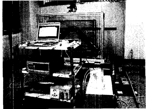
Fig. 4. Photograph of burst test for local wall-thinned elbow.
