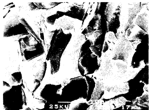
Fig. 11. Cleavage fracture surface of the fatigued gray cast iron.
