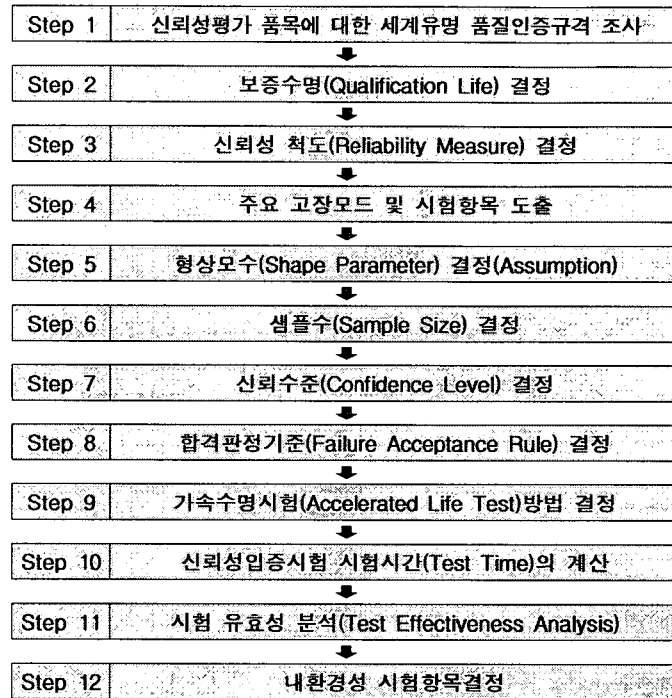
Fig. 7 Procedure for reliability substantiation test of mechanical components
