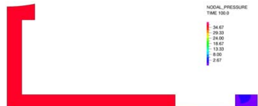
Fig. 4 Nodal pressure contour in fluid domain (p=35MPa)
