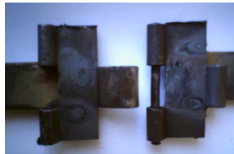
Fig. 8 Shape of Tensile strength test of hinge belt plate(forming type)
