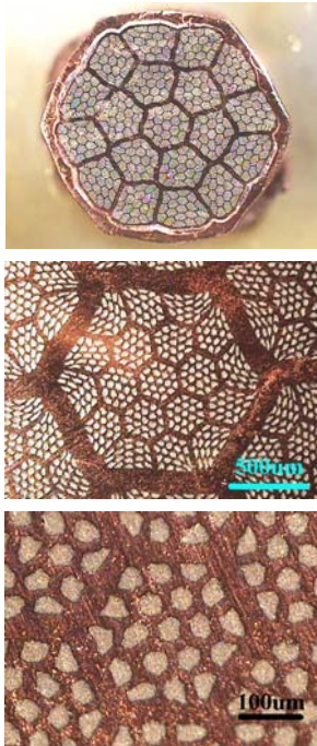
Fig. 7 Section of 19x19 filament wire (width of filament : 33µm)
