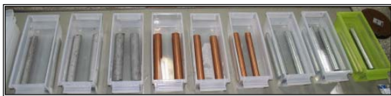
Fig. 2 Immersion form of piping material
