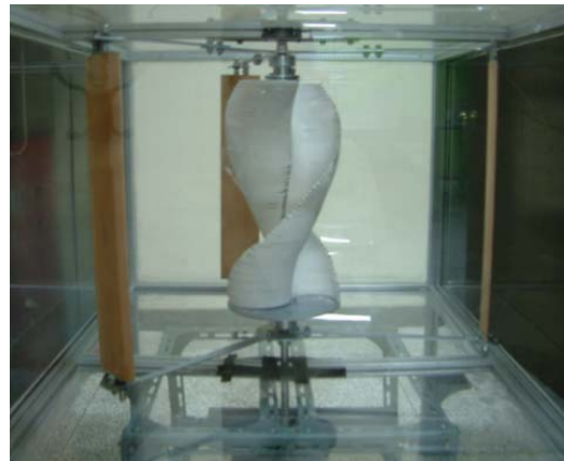
Fig. 10 Combined helical Savonius and Darrieus turbines fitted inside the wind tunnel
