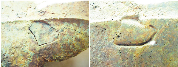
Photo 3. Traces of the hole in the casting mold.
