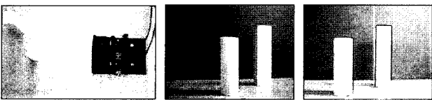
FIG. 6. Case 3: the objects are located at (0,350), (100,450). (a) the object's position (b) left image on the left CCD (c) right image on the right CCD.
