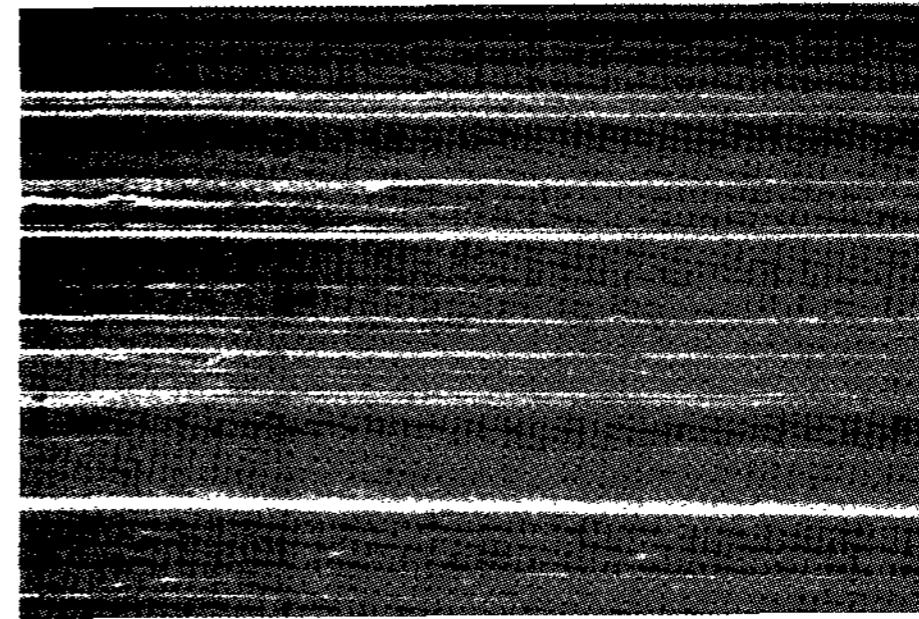
**Figure 6.** Test specimen. Pure titanium machined surface conditioned with 50mg/ml tetracycline-HCl for 2½min( $\times 2,000$ ). After treatment, machining line is more pronounced for the control specimen. But in general, test specimens are similar to control.
