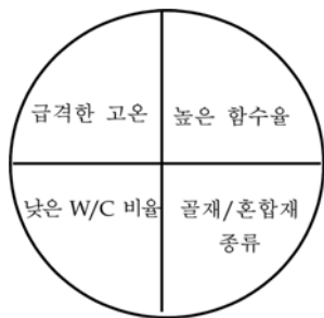
Fig. 2. A schematic of spalling phenomenon condition.
