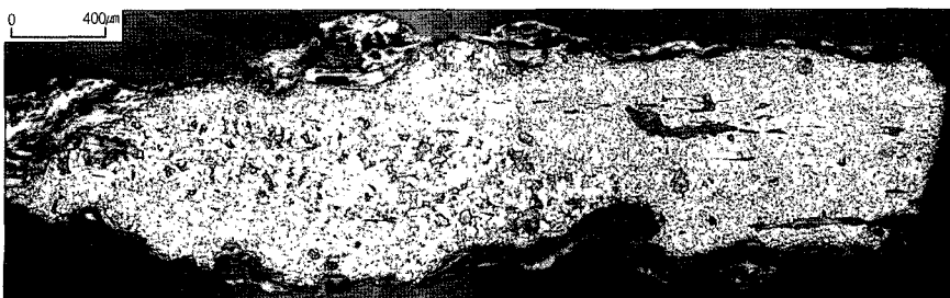
Figure 10. Microstructure of 'a' (vertical section) of Iron axe.
