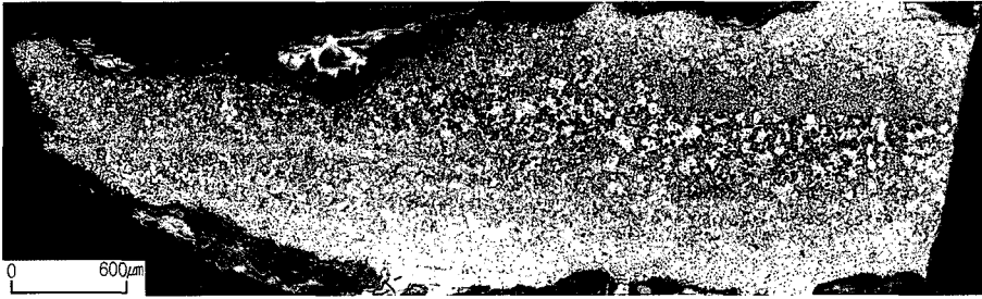
Figure 24. Microstructure of 'a' (vertical section) of Iron sword.
