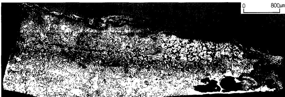
Figure 12. Microstructure of 'b' (vertical section) of Iron axe.
