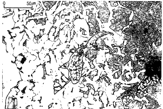
Figure 44. Microstructure of vertical section of Iron spear.
