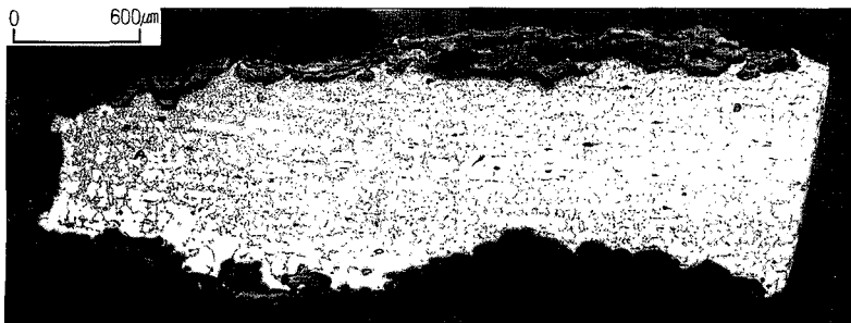
Figure 30. Microstructure of 'c' (cross section) of Iron sword(X50).
