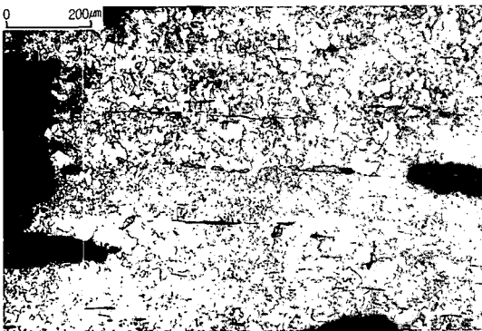
Figure 47. Microstructure of cross section of Iron sickle.
