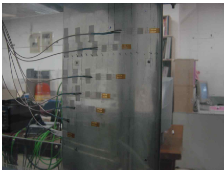
Fig. 4. Glue-on probes on airfoil surface
