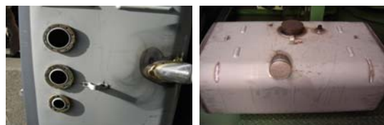
Fig. 2 Steel fuel tank(used seam, CO 2 +Ar weld method)
