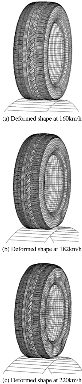
Fig. 12 Standing wave phenomena of the pattern tire model
