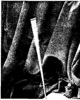
Fig. 5 One to one resonance of the circular cantilever beam on the first mode
