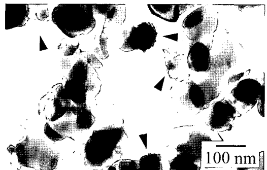
Fig. 1. TEM image of the Al_2O_3/5 \text{ vol\%} Cu powder mixture after hydrogen reduction at 350^\circ\text{C} for 30 min.
