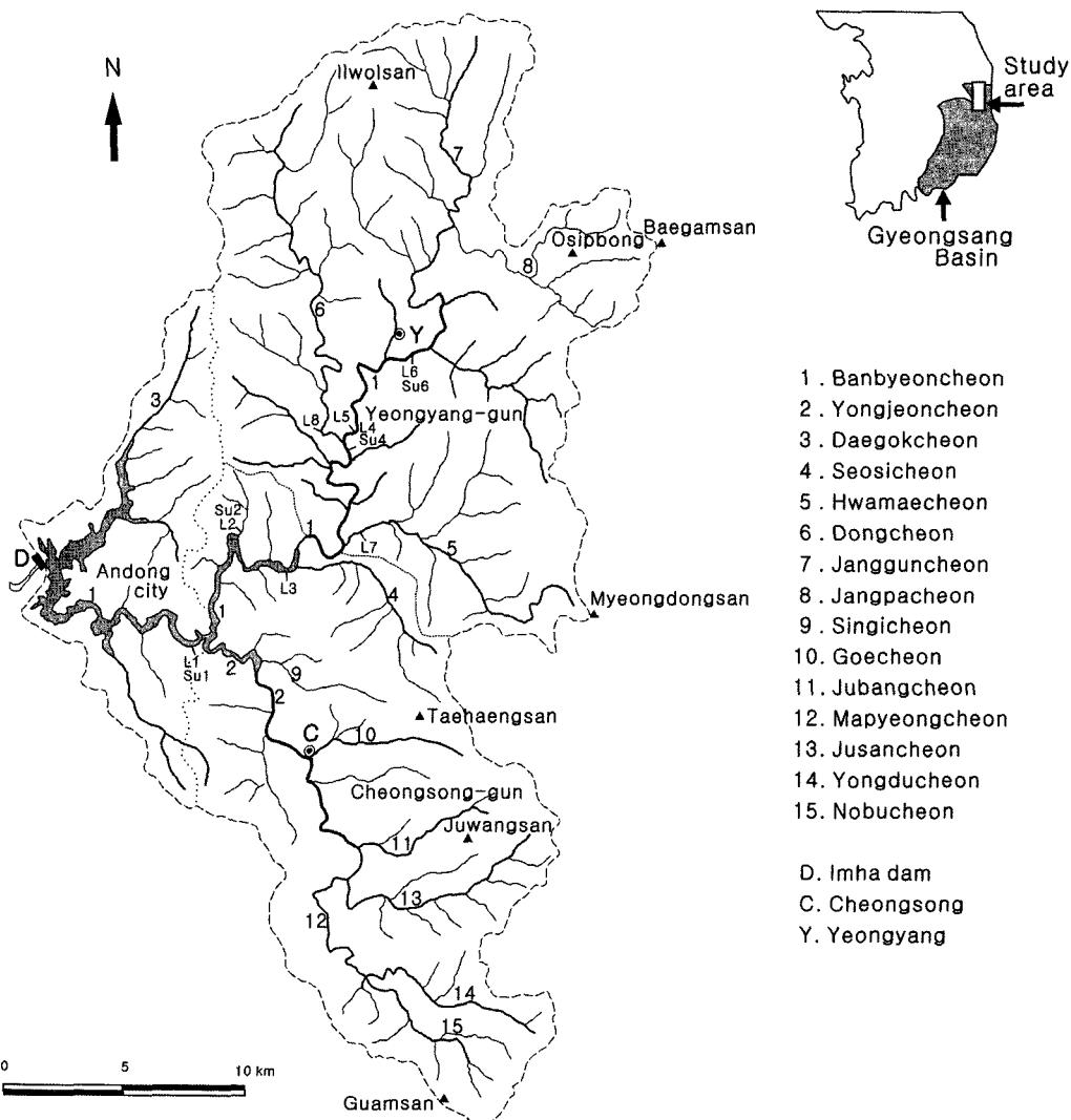
**Fig. 1.** Map of water system in drainage field of the Imha dam, showing locations drawing turbid waters and measuring their turbidity.
