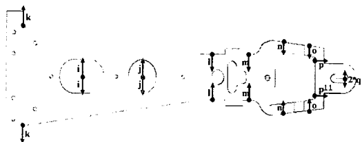
(b) Design parameters of load-beam
