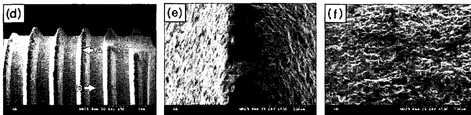
Fig. 2. SEM showing the surface morphology of SA non-treated and SA treated Ti-6Al-4V implant. (a),(d) implant shape, (b),(e) crest surface at A point, (c),(f) valley surface at B point.
