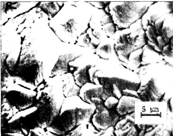
Fig. 6. Top ceramic coating of EB-PVD TBC before oxidation test.
